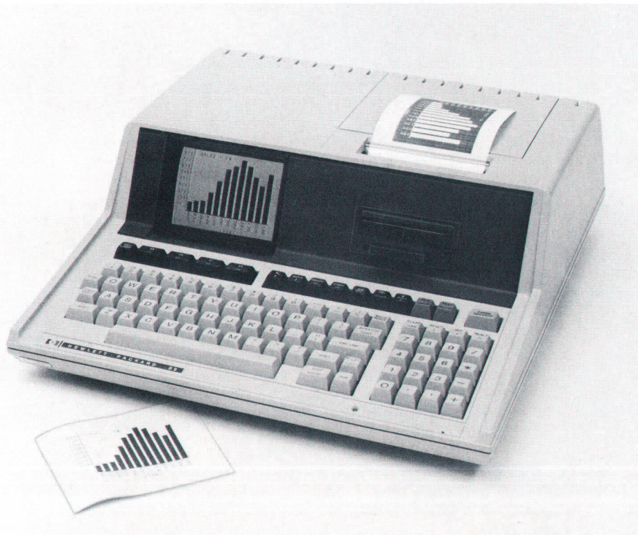
Fig. 1. The HP-85 Personal Computer uses BASIC language programming and operating commands that are permanently resident in the system firmware. Contained in a single package are all of the elements for a small computer system—keyboard entry, tape mass storage, CRT display, and a thermal printer. The inverse video display mode is shown with the associated printer copy at the upper right. In the left foreground is the printer copy for the normal white-on-black display mode.
